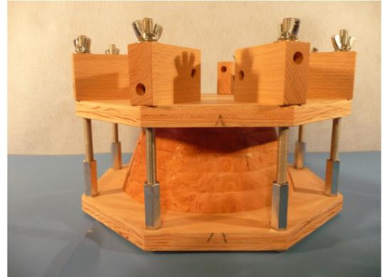
The photo to the right shows that with the addition of eight more coupling nuts the press can now handling pieces up to 18" tall. Here the press is used to clamp a 15" tall project.
